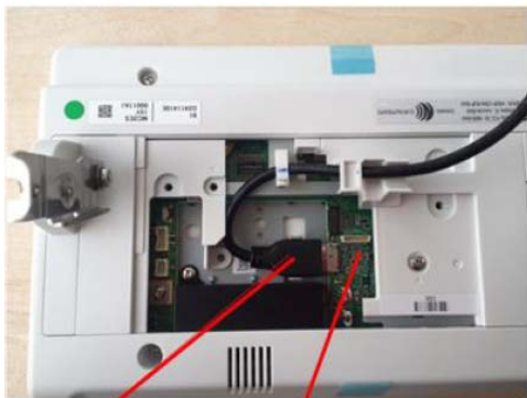
CABLE: OPERATION SUB-UNIT:USB3.0 PCB:SUB:PROGRAM:ASS'Y
