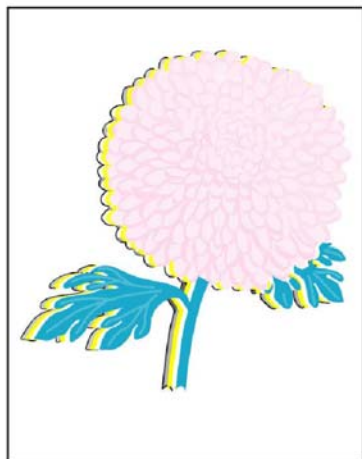
Figure 1 Color reg misalignment
